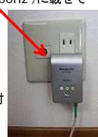
A photograph of a white PLC modem plugged into a standard Japanese power outlet. A red arrow points from the text 'PLCモデム' to the device.
